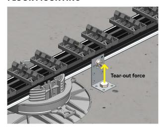
Use an angle bracket or steel strip with M6 bolts to anchor the deck to the ground. Fastening is staggered, and the number of anchors per  $m^2$  can be determined by taking into account the uplift force due to wind and the deck's own weight.
